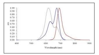
**Figure 1.** Normalized absorbance (grey), excitation (blue) and fluorescence emission (red) spectra of *Cat K 680 FAST* in 1x PBS.
